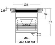
Soft silicon seal holds the fitting into the cut-out
